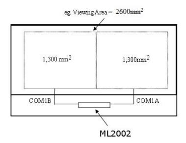
Note: COM1A and COM1B shall cover half of the Viewing Area (ie. Area = 1,300mm<sup>2</sup>) Each Common shall not connect to each other.
